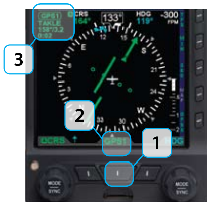
Figure 4-56 Navigation Source Information Block
