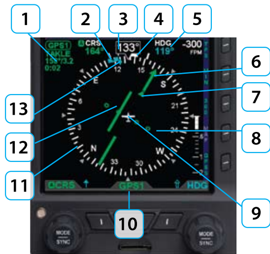
Figure 4-32 Horizontal Situation Indicator
